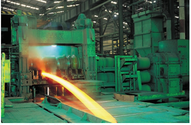
3 Merdaneli Kaba Haddeleme Makinesi
